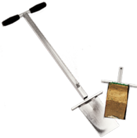
Soil Profile Sampler A robust shovel type sampler, slightly tapered to give a clean cut with minimal disturbance. The blade is easily removed to allow examination of the profile. The plug can be replaced with minimal surface disturbance.
