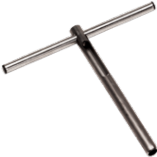
Handy Stainless Soil Sampler A high quality small core sampler (3/4" 2cm) manufactured in stainless steel and features a double window tine for quick and easy appraisal of soil stratas near the surface. This handy sampler has a loose 'T' handle for convenient storage, and for assistance with removal of the sample. Supplied complete with storage container.
