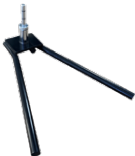
Car Base 'V' shape allows base to be wedged under any parked vehicle wheel (or driven onto).
