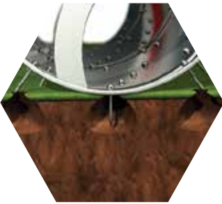
Cross section showing shape of incision made by spikes.
